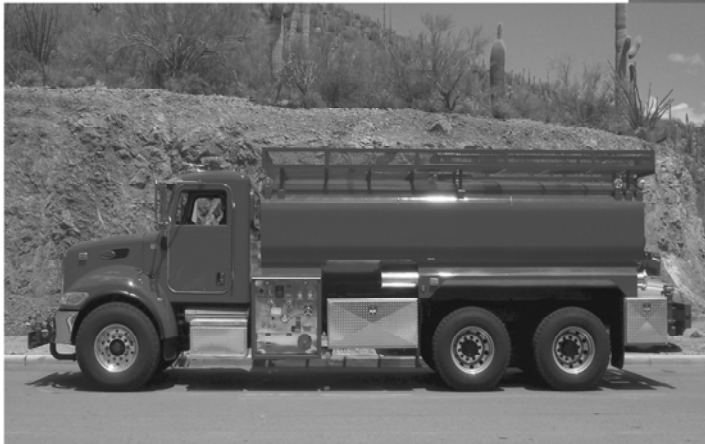
4,000 Gallon Hot Dipped Galvanized Steel Tank
